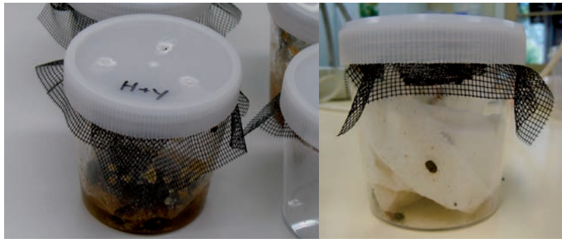
Figure 5. Attractant trap used to trap emerging adult SHB in field trials. Trap with honey and yeast mixture before it was added to an enclosure (left); trap with added crumpled paper and adult SHB after removal from enclosure (right)
